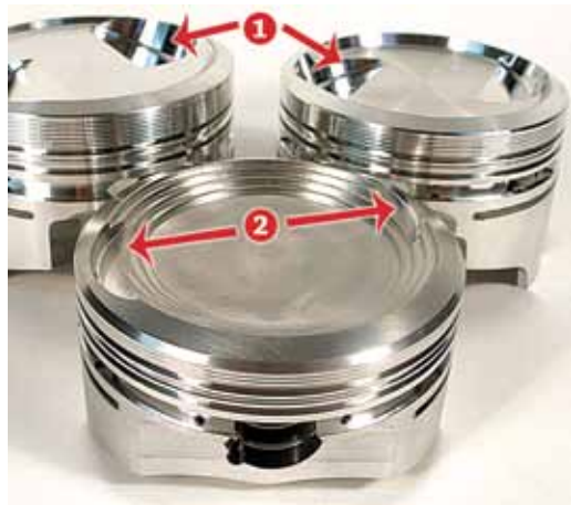
Far top left is our 2900 Sport Piston with our 3200 Sport Piston shown top right. Both have deep valve pockets to protect them from the valves in the event of a cam belt failure. Front and center is our 3200 Rally Piston with shallow valve pockets.
