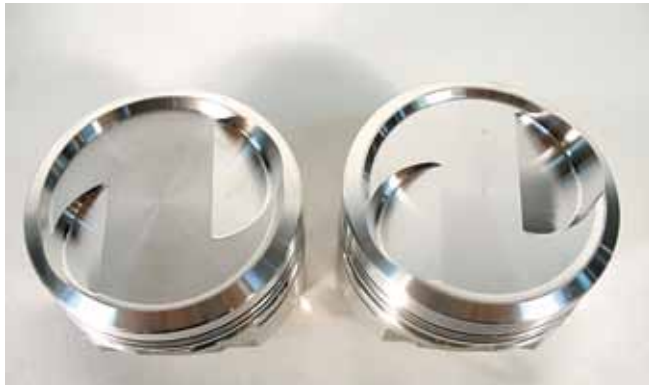
Left: MM 3200 Sport Piston & Right: MM 2900 Sport Piston Both with deep valve pockets.
