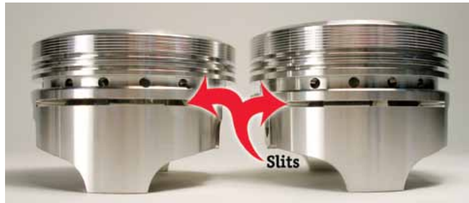
Left: 3200 Sport Piston. Right: 2900 Sport Piston. Notice the horizontal slits just below the oil ring groove. Slits prevent piston crown heat from directly transferring to the skirt, consequently reducing piston expansion to only 5% over that of a stock cast piston. Also allows oil feed into the top of the skirt which prevents scuffing.
