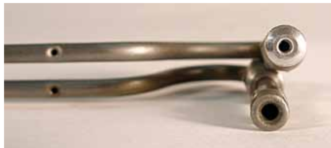
Bottom: Stock Sprayer Bar has a .110" oil feed hole into the bar. Top: MM Sprayer Bar with a .062" oil feed hole to prevent oil build-up in the head at higher rpms and under track use.
