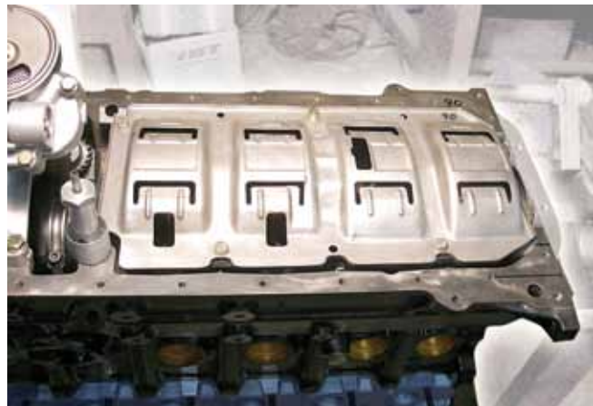
MM Windage Tray with Scrapers - used to remove oil spray from the crank.
